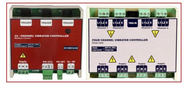
ECVIB12 produce a highly stable output voltage that is adjustable in from 1% to 99%. Thanks to the soft-start output, the feeder starts quietly and ensures gentle product handling. An on-board fuse provides over current protection for the feeder coil as well as for the internal semiconductors. Power LED indication available.
